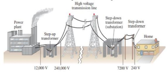
At generating station, normally voltage is stepped up to around thousands of volts. Power losses increase with the square of current. Therefore, keeping voltage high current becomes low and the loss is minimized.
